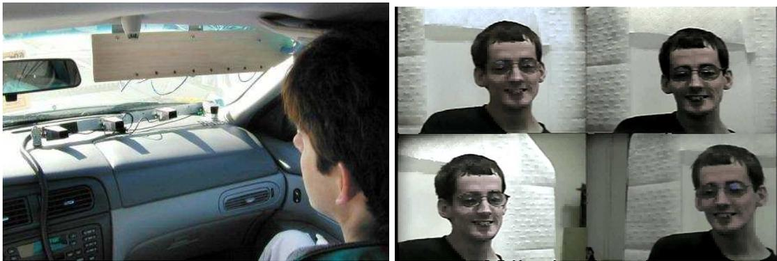
Figure 1: Left image shows the AVICAR transducer array deployed in an automobile: four cameras (on dashboard), eight microphones (embedded in wooden baffle, at level of the sunvisor). Right: the image of one dysarthric subject, acquired by deploying the AVICAR array on top of the monitor of a personal computer.
